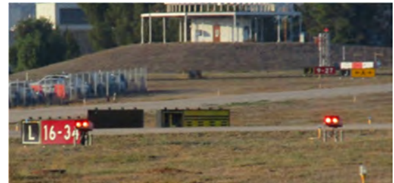
Two-Light Precision Approach Path Indicator (PAPI-2)
